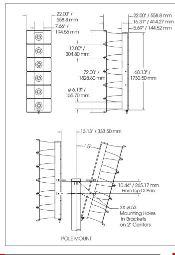
Color: Black projectors with Off-White Housing Paint:TGIC - Polyester Powder Coat, highly corrosion resistant Frequency Response: 200-2000Hz
